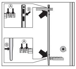
The washing machine must not be moved without the transit bars in place.
